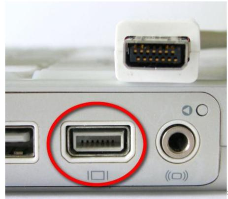
**Mini-DVI:** Replaced Mini-VGA on the PowerBook G4, iMac, MacBook, and 2009 Mac Mini. Mini-DVI does not support dual-link connections and cannot support resolutions higher than 1920x1200 @60Hz.
